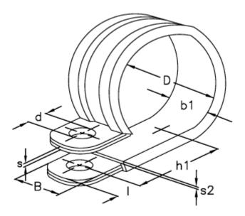
$\begin{array}{lll} \text{b1} & = 25.0 \\ \text{d} & = 8.4 \\ \text{Diameter D} = 75 \\ \text{h1} & = 52.0 \\ \text{I} & = 8.5 \\ \text{s} & = 0.80 \\ \text{s2} & = 2.0 \\ \text{Width B} & = 20 \\ \end{array}$
